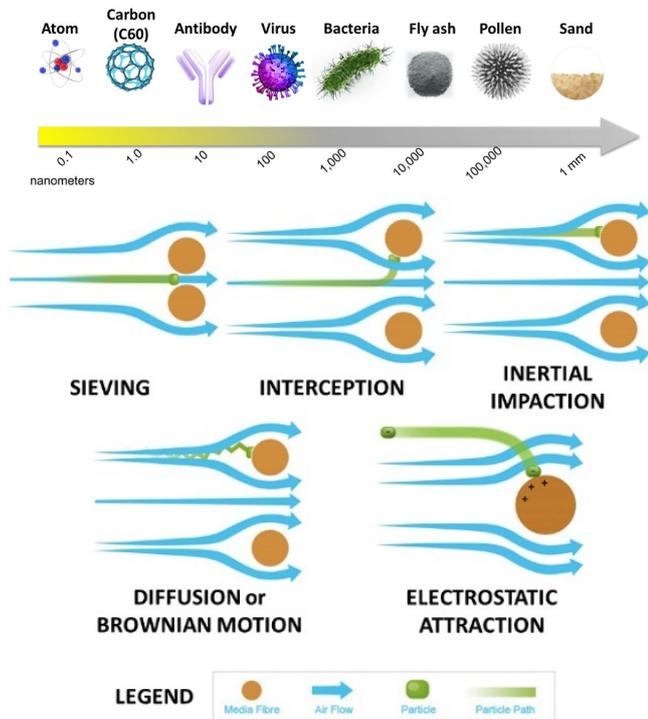
**Figure 2:** Concept of size of particles present in nature (top),[9] and the mechanism associated with mask filters (bottom).
