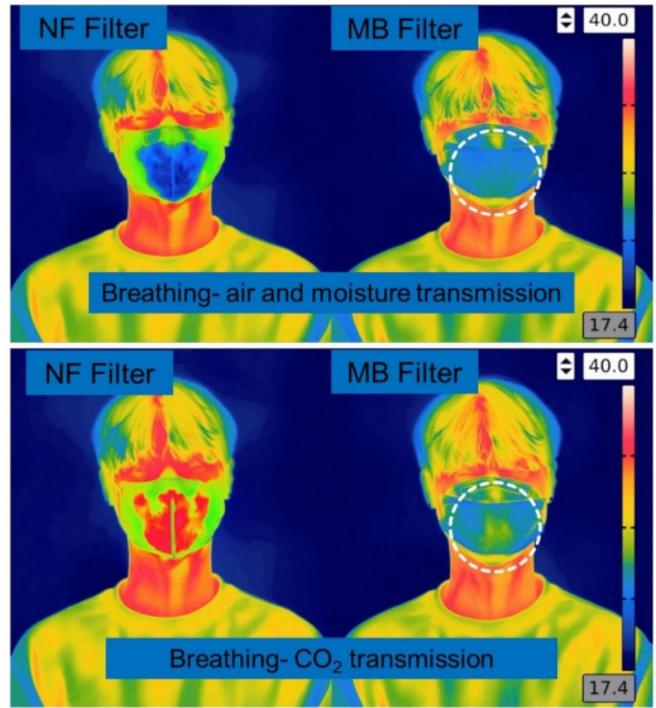
**Figure 4:** Evaluation of breathing comfort by infrared thermal camera of ES NF filter and MB filter: (top) air and moisture transmission and (bottom) CO<sub>2</sub> transmission. Figure from reference.[15]
