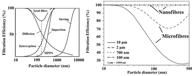
**Figure 3:** Filtration efficiency as a function of particle diameter for single-fibre mechanisms and total filtration efficiency (left).[13] Filtration efficiencies of four fibrous filters with different fibre sizes (right). Figure from reference.[14]
